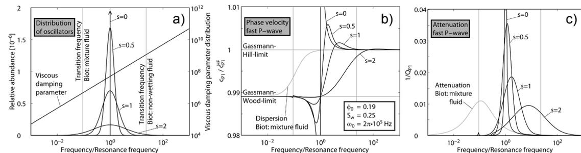
Figure 3. Frequency dependent phase velocity  $c_{P1}$  (b) and inverse quality factor  $1/Q_{P1}$  (c) of the fast P-wave for different distributions of fluid blob sizes  $c(\omega)$  and damping coefficients  $\alpha(\omega)$  shown in a).
