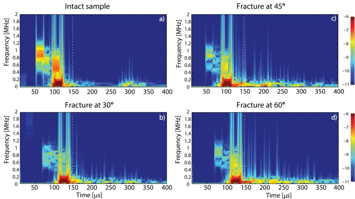
Figure 4. Spectrograms of receiver time signals generated by an S-wave with a source frequency of 1 MHz propagating through the intact sample (a), and fractured samples with a fracture inclination angle of 30° (b), 45° (c), and 60° (d), respectively.
