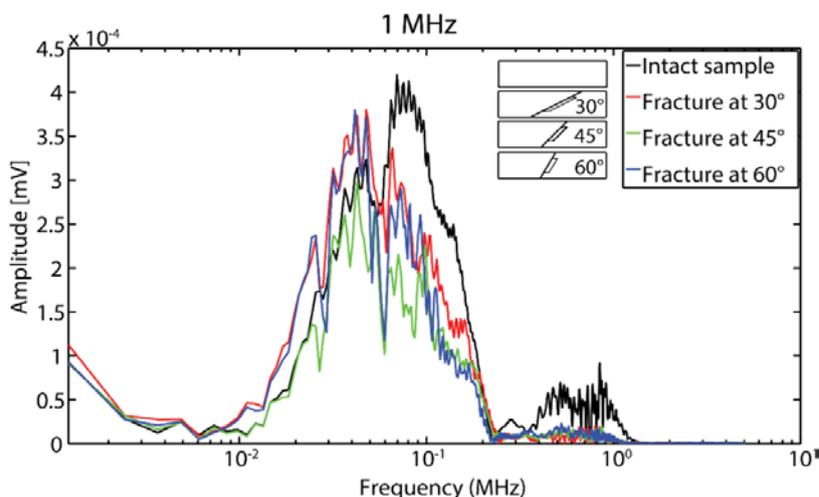
*Figure 3. Receiver spectra for experiments with a dominant S-wave source frequency of 1 MHz for the intact sample and fractured samples with a fracture inclination angle of 30°, 45°, and 60°.*
