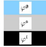
Concept of phenomenological continuum-mixture theory. Individual fluid surfaces disappear during the superposition of the three continuum fields.
