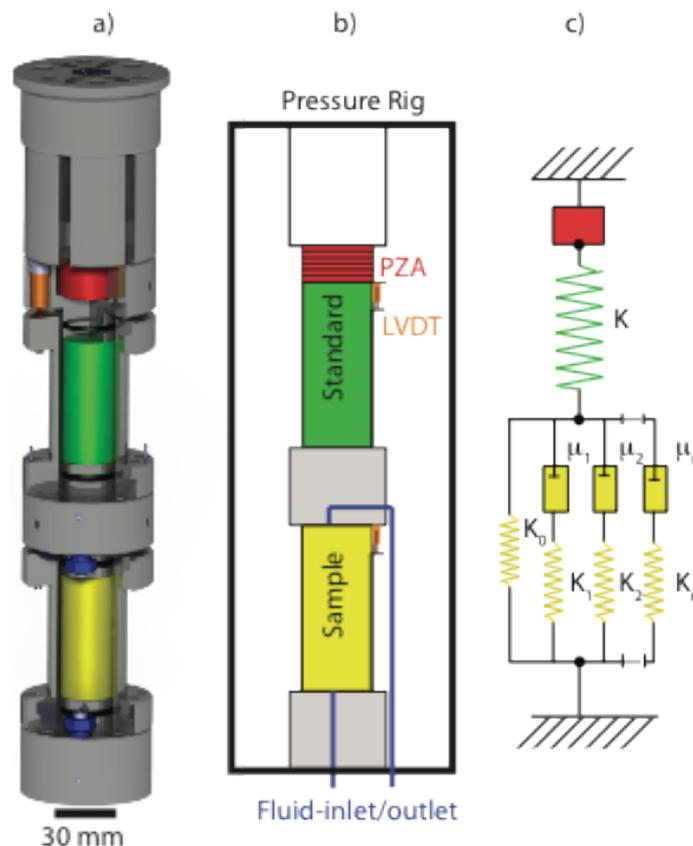
Figure 1. Schematic cross-section of the ETH-developed SWAM (Madonna et al. 2011). a) CAD drawing, b) Sketched construction, c) Physical model.
