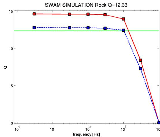
Figure 2. Results of the SWAM computer experiments for a Rock sample with an attenuation of  $Q=12.33$  (green line) for a range of applied excitation frequencies.  $Q_{\text{real}}$  (red solid line) can be compared with the real experimental setup. An optimized sensor positioning allow for more accurate measurements of  $Q$  ( $Q_{\text{opt}}$ ; dashed blue line).
