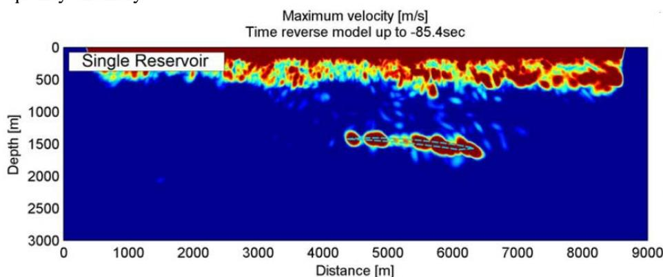
**Figure 3** Distribution of maximum velocities in reverse modeling simulations. Shown is the result of a numerical feasibility study with the focus on microtremor localization.
