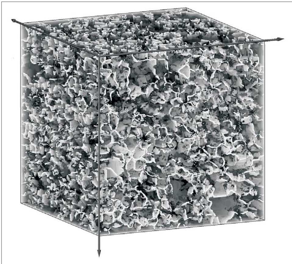
Figure 4. Micro-CT image of the Berea sandstone sample after watershed segmentation. The grain contacts identified by the watershed segmentation are shown. The cube volume is 2 \text{ cm}^3 .
