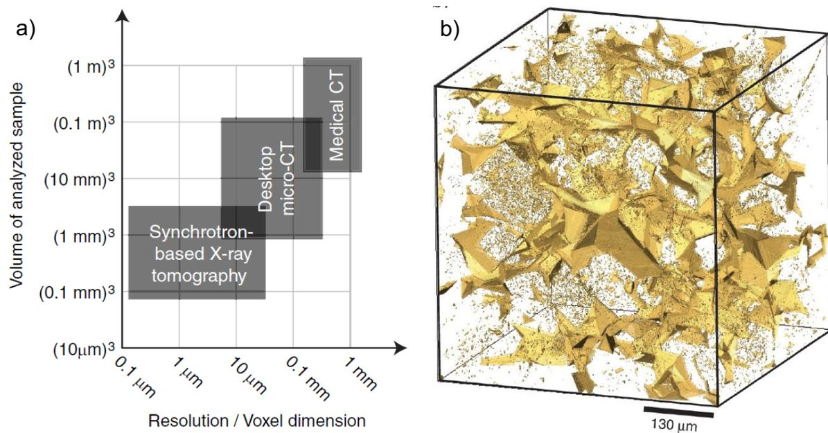
**Figure 1** a) Schematic representation of sample size versus resolution of the most common X-ray computed tomography methods. Other methods are available, but are not plotted here. b) 3D visualization of the SRXTM-volume of dry Fontainebleau sandstone. Only the pore space is shown in yellow; the quartz grains are not shown.
