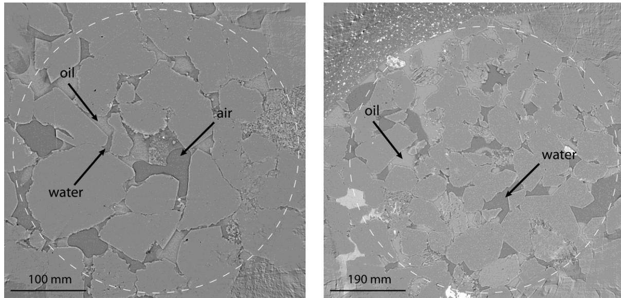
**Figure 2:** Raw SRXTM-images of Berea sandstone partially saturated with water, air, and oil (left) and with water and oil (right). The full data cubes contain  $1024^3$  voxels each with a voxel size of  $0.38 \mu\text{m}^3$  (left) and  $0.74 \mu\text{m}^3$  (right).
