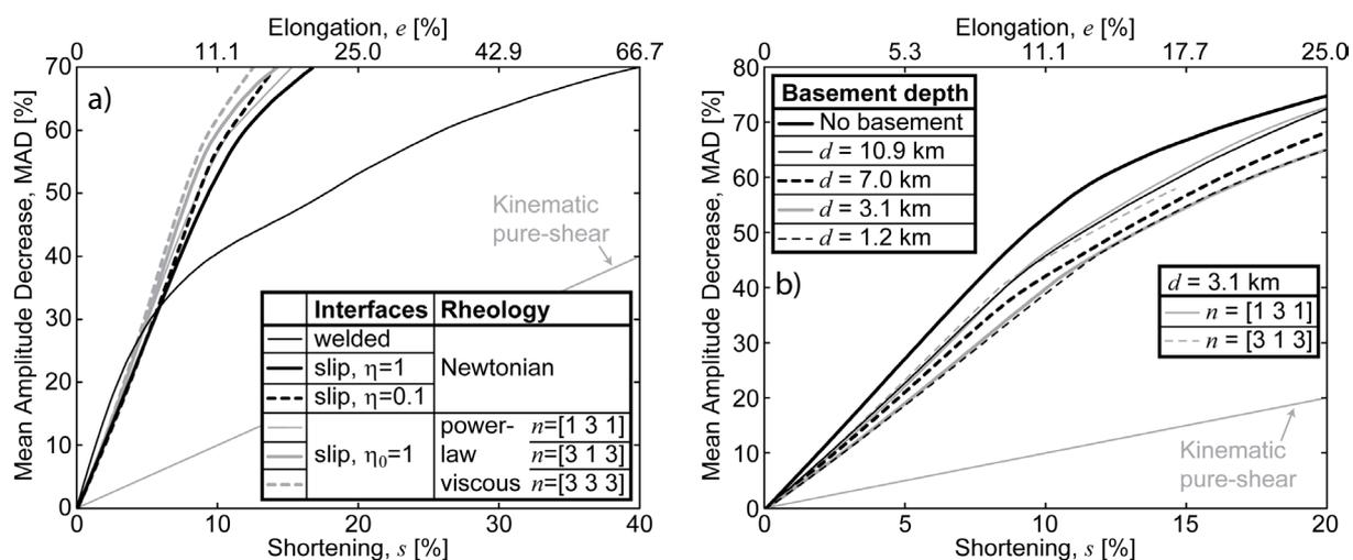
Figure 2: Mean Amplitude Decrease during different progressive dynamical unfolding simulations (a) without and (b) with a basement at depth  $d$ . The bold black line is the same in (a) and (b). The legend in the upper-left corner in (b) corresponds to simulations using a Newtonian rheology; the second legend corresponds to simulations using power-law viscous rheologies. Kinematical pure-shear is equivalent to dynamical unfolding with no mechanical difference between the layers ( $MAD=s$ ).
