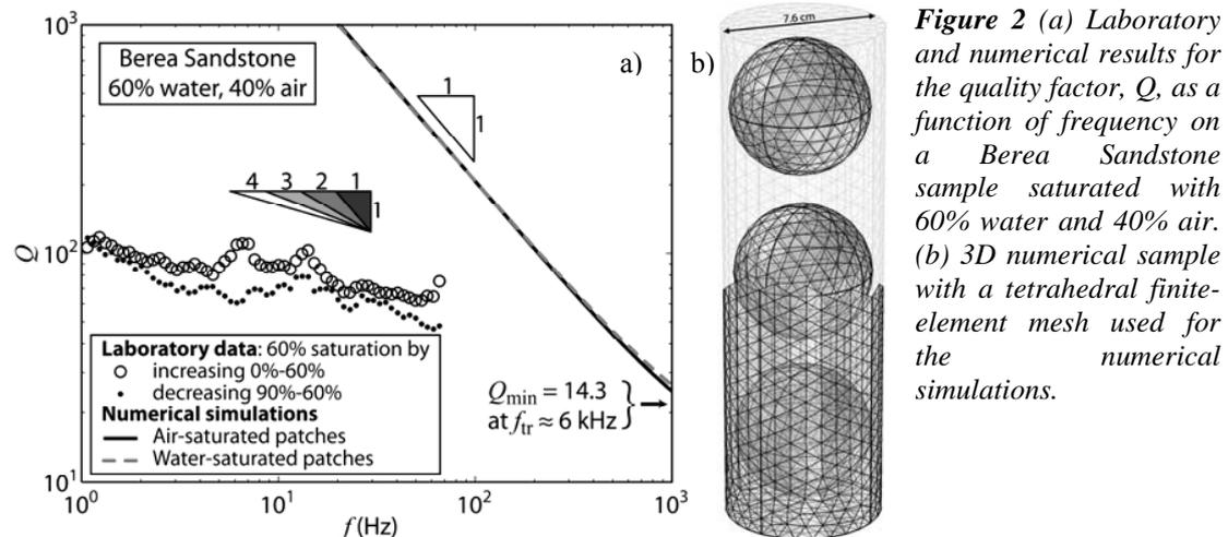
**Figure 2** (a) Laboratory and numerical results for the quality factor,  $Q$ , as a function of frequency on a Berea Sandstone sample saturated with 60% water and 40% air. (b) 3D numerical sample with a tetrahedral finite-element mesh used for the numerical simulations.
