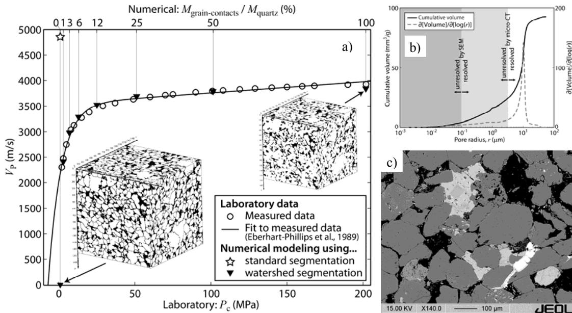
**Figure 1** (a) Laboratory and numerical results for the P-wave velocity,  $V_P$ , at 3 MHz as a function of confining pressure,  $P_c$ , in a Berea Sandstone sample. (b) Mercury porosimetry measurements. (c) Scanning Electron Microscopy (SEM) image.
