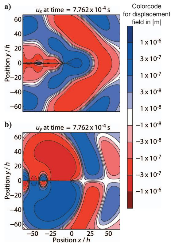
Figure 11. (a) Snapshots of the  $x$ - and (b)  $y$ -component of the 2D displacement field of a simulation of an SGW propagating along an elliptical crack (second model in Figure 1). The crack is filled with viscous oil and has a small gas cap at the crack tip. Contour lines are the same as in Figures 6 and 7. Axis labels for the abscissa are only given in (b) but are valid in (a) also.
