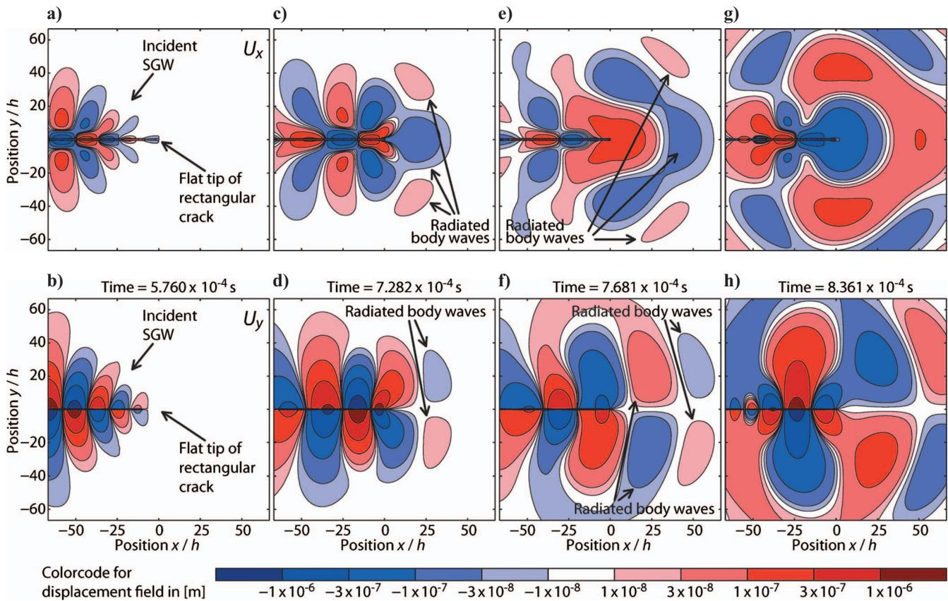
Figure 7. Same as Figure 6 but for a rectangular crack with a flat crack tip (third model in Figure 1). Note that the time of the snapshots is not the same as in Figure 6 because the SGW travels with a slightly different velocity.
