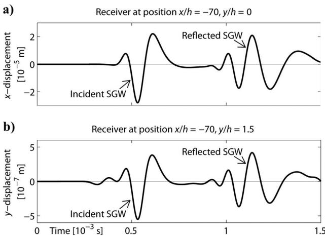
Figure 8. (a) Displacement-time signal in the  $x$ -direction at a receiver inside the crack on receiver line 1 (Figure 1). (b) Displacement-time signal in the  $y$ -direction at a receiver outside the crack on receiver line 1. Both traces are obtained from a simulation of an SGW propagating along an elliptical crack (second model in Figure 1) filled with viscous water. Labels for the time axis are only given in (b) but are valid for (a) also.
