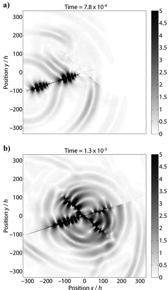
Figure 12. (a and b) Snapshots of the 2D displacement field at two different points in time of a simulation of an SGW propagating along an elliptical crack that is intersected by a second elliptical crack. The displayed value is the normalized absolute particle displacement  $10^6 \sqrt{u_x^2 + u_y^2}$ . The cracks are filled with viscous water. Axis labels for the abscissa are only given in (b) but are valid in (a) also.
