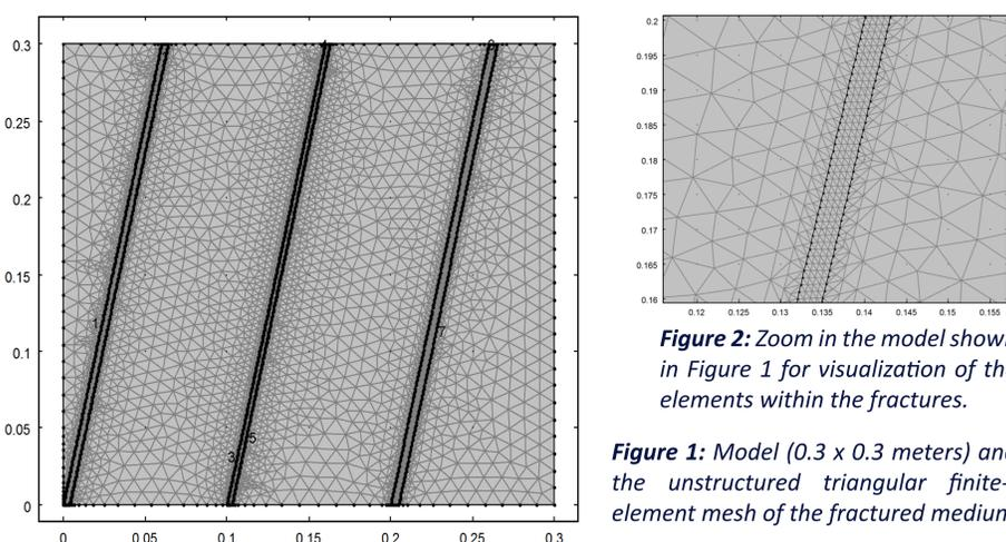
Figure 2: Zoom in the model shown in Figure 1 for visualization of the elements within the fractures.
